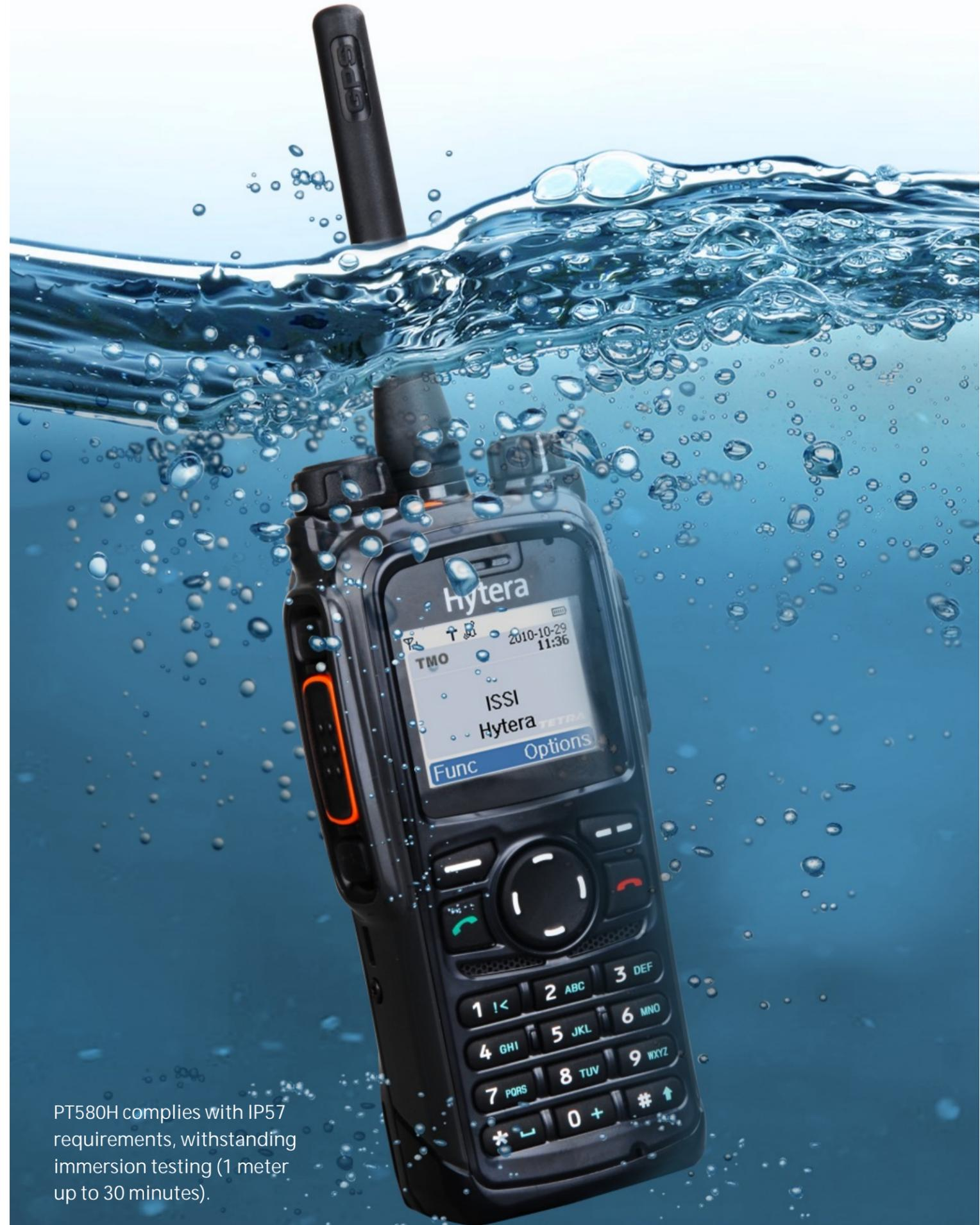
PT580H complies with IP57 requirements, withstanding immersion testing (1 meter up to 30 minutes).
